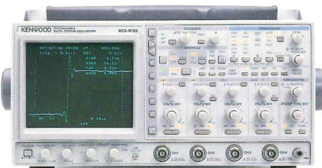
DCS-9120 (40MS/s simultaneous 2ch) 16K word/ch memory 100MHz 4ch real time
